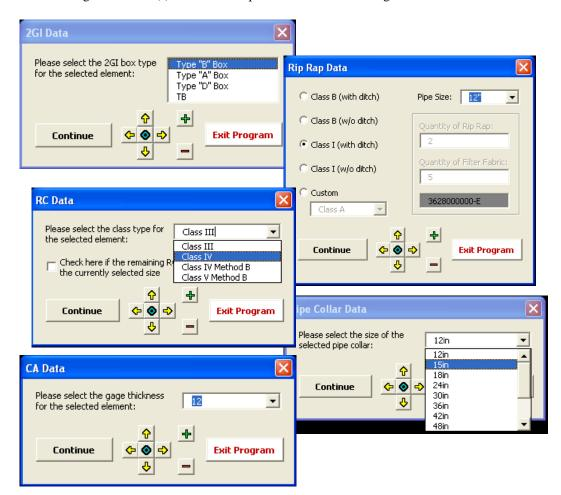
Included on each dialog box is a series of navigation buttons. While the VBA is running, Microstation commands are unavailable. Since the user may need to zoom or move within the drawing to determine information necessary to complete the Adhoc, these buttons were included on each dialog. The green button located in the middle of the four pan buttons is used to bring the current feature back to center.
